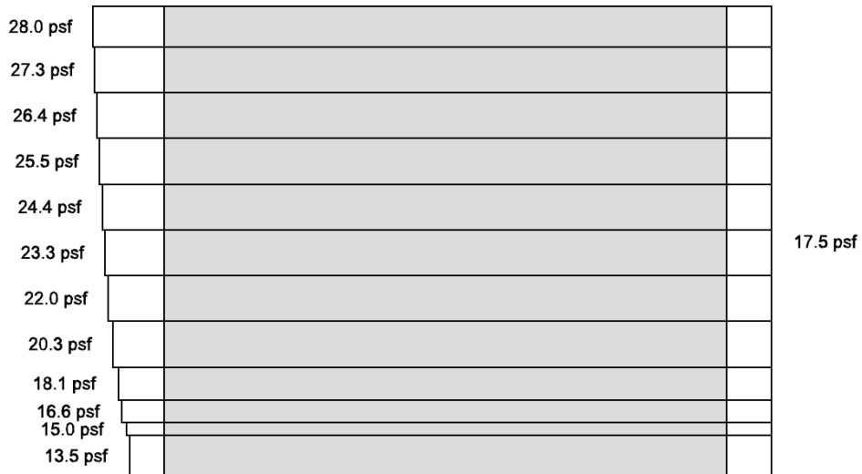
Figure D – Wind pressure diagram for East-West direction
